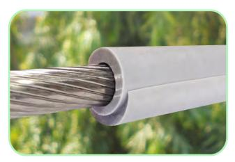
Gala Silicon Overhead Line Covers are made from high quality non-tracking silicon rubber that are designed for field installation over bare conductors. These covers provide a layer of electrical insulation for Phase-to-Phase and Phase-to-Ground protection from bird and animals. The GSOC provides electrical insulation, UV resistance and tracking resistance. Silicon Self-fusing Tape can be applied on it for better insulation.
